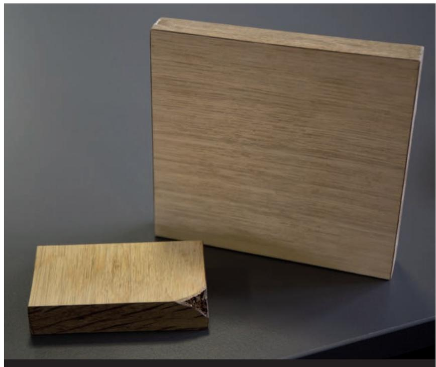
The fibres in the chopped and dried bark can be pressed and shaped to form a kind of chipboard. This can then be covered with wood or linoleum.
