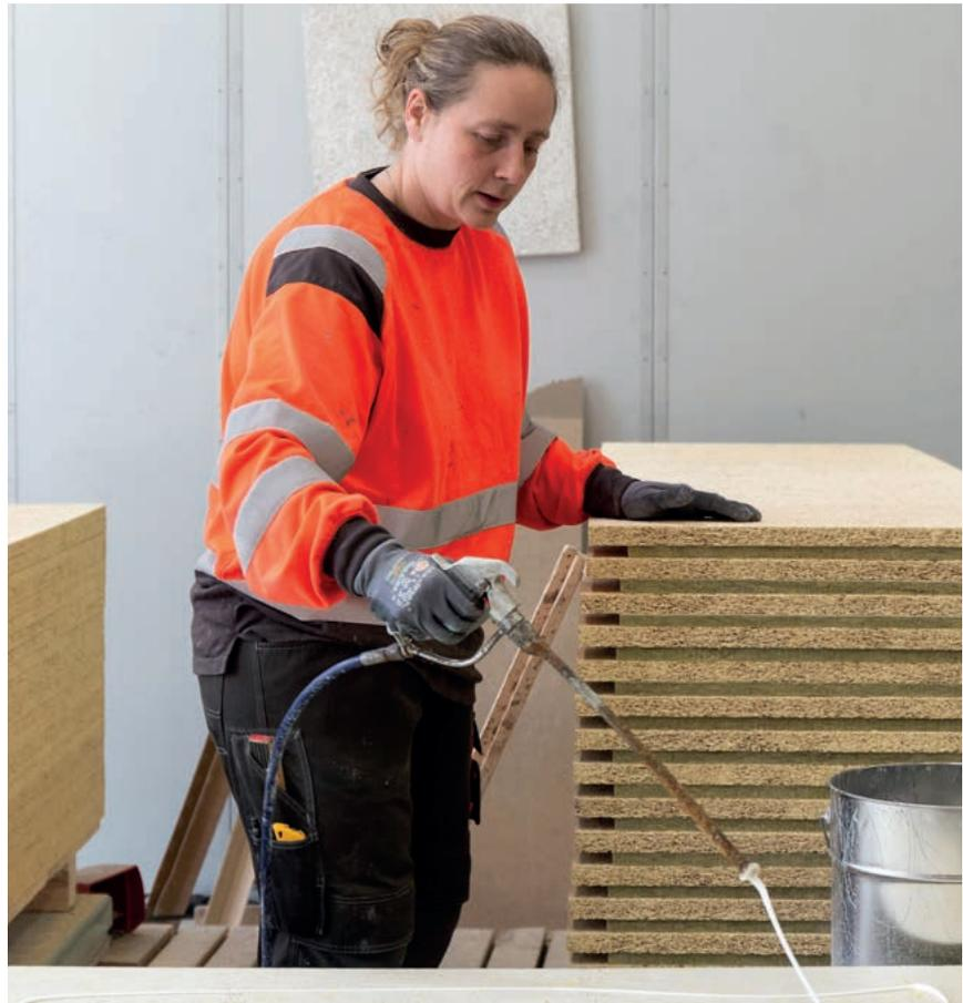
cut out insulation and glued it on to the acoustic panels. Unlike some of the factory's other departments, the pace is not as high in the carpentry workshop, and therefore the permanent employees have more time to provide support and impart their knowledge.
