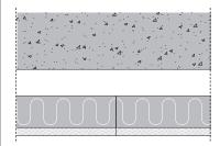
Here, too, a suspended Troldtekt acoustic ceiling has been installed beneath the concrete ceiling. The structure consists of classic 25 mm Troldtekt acoustic panels and 95 mm mineral wool above. With a gap above the mineral wool, the total installation height is 200 mm.
