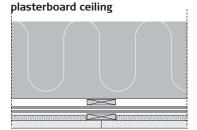
Here, Troldtekt acoustic panels have been retrofitted beneath the plasterboard ceiling. The Troldtekt Plus acoustic panels are two-layer panels with a mineral wool backing.
