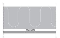
In the example, two layers of plasterboard have been used to ensure an attractive finish. One layer of plasterboard is also a popular solution, although it does not make much of a difference for the acoustics.
