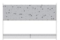
Here, a suspended Troldtekt acoustic ceiling is installed beneath the concrete ceiling. The Troldtekt Plus acoustic panels are two-layer panels with a mineral wool backing. With a gap above the Troldtekt ceiling, the total installation height is 200 mm.
