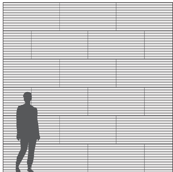
Troldtekt line installed horizontally
