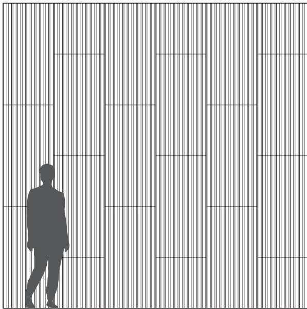
Troldtekt line installed vertically
