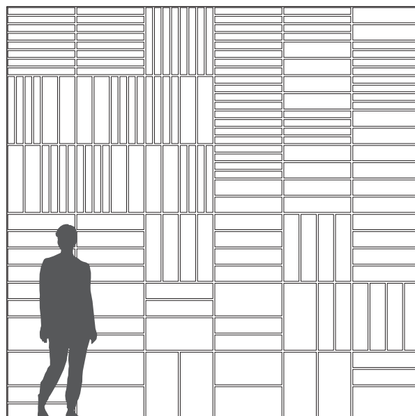
Troldtekt tiles randomly installed
